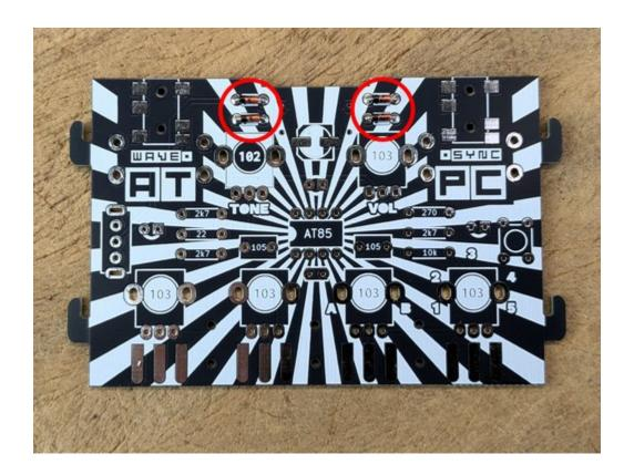
The resistors can now be soldered in. These resist the current flow and limit it. For them, the direction does not matter.
