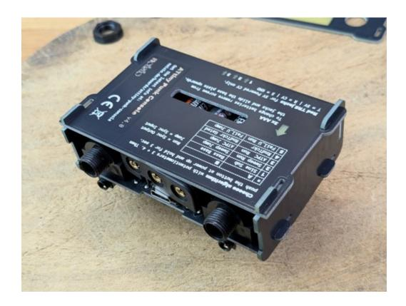
Finally, the plate with the ATPC lettering can be attached to the **back** and the housing can be completed by fastening the **2 nuts**.
