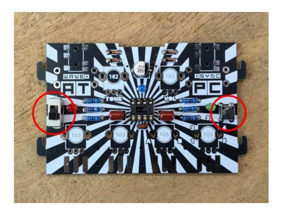
This is followed by the two **black 3.5mm jack sockets** on the top. The SMD technique should be used here again, where only a single soldering point is set first.
