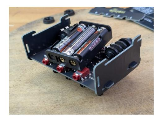
The next step is to insert the **front panel**. The two side panels must be **bent slightly outwards** and the panel pushed in from above.
