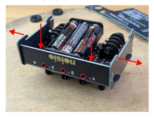
The **base plate** is now installed and pushed forward until it is in line with the front panel.
