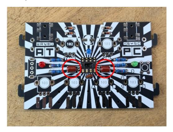
In **some of the following steps**, **SMD components** are now installed on the board surface. For some, it is important to align them precisely. This ensures that the sockets, for example, fit well into the housing later.
