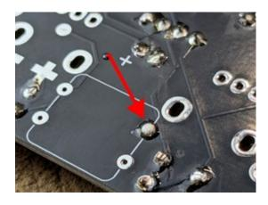
This can now be tried out on the top side with the 220uF capacitor. It must be positioned according to the marking. First just place a soldering point > align > finish soldering.
