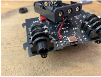
In **version B**, note the **different position of the two pads** to the left and right of the USB socket.
