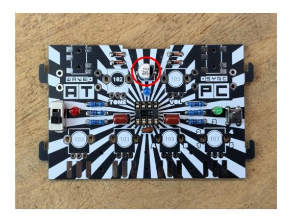
Attention: In a slightly revised  $version\ B$  of this PCB, this  $capacitor\ is\ rotated$ by 180°. Please follow the current marking on the board.
