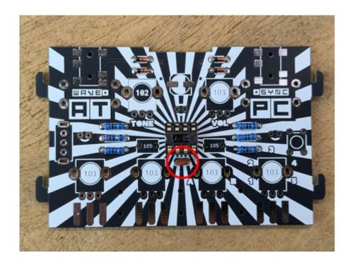
Next, the **LEDs**. From left to right: RED - BLUE - GREEN. Again, **the direction must be observed** when inserting.
