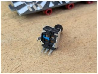
To get the **potentiometers well aligned**, you should first solder only the middle one of the three legs and correct it if necessary.
