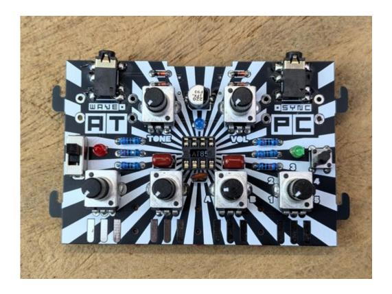
The 6.35mm sockets can then be installed from below and soldered on the upper side. Make sure that the legs are well inserted and that the ends are sticking out by just about 2 mm.
