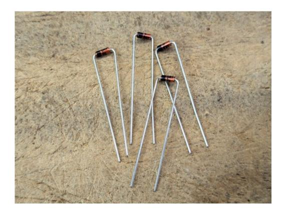
After insertion, the legs of the THT components can be **bent slightly outwards**. This prevents them from falling out again.
